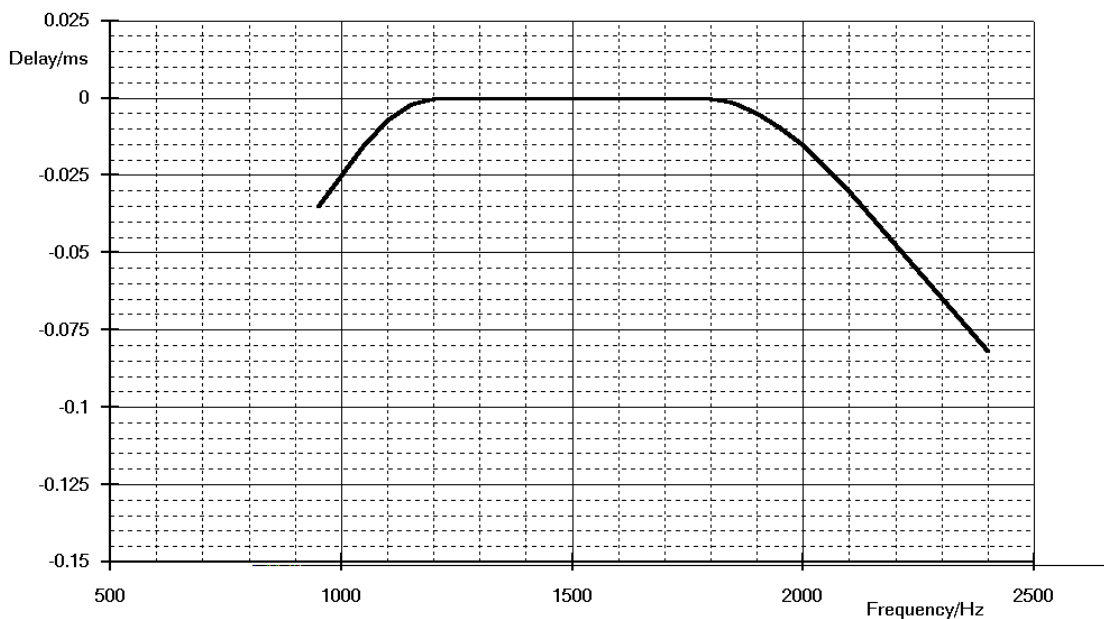
Figure 3 Rx Equaliser Group Delay (RXEQ = '1') with respect to 1700Hz
